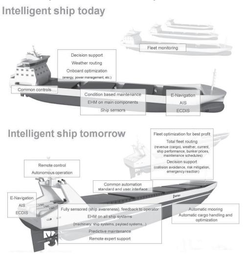
Figure 1.5. Towards the autonomous ship of the future
